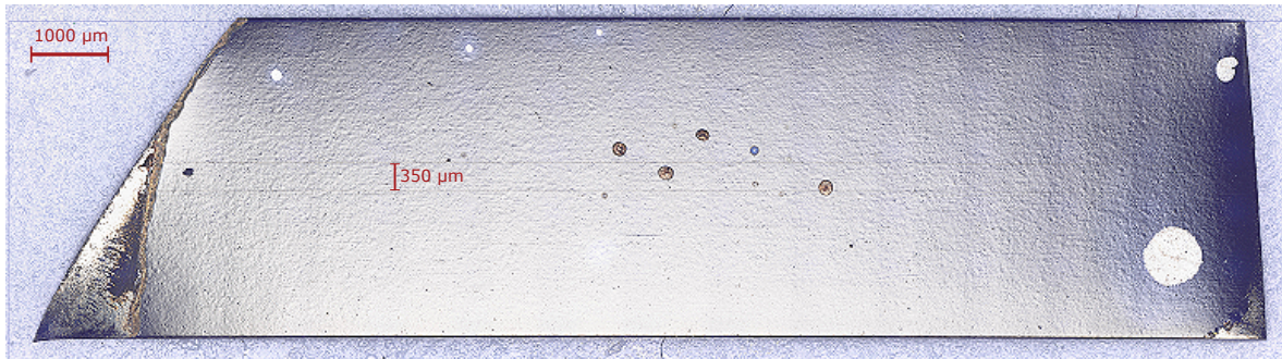
Figure 6.18 – Picture of a representative position in the defect zone of tape #T-2 taken via light microscope. Copper and silver have been etched and two parallel, \sim 1 \mu\text{m} thick scratches, separated by 350 \mu\text{m} are visible in the YBCO film. This scratch blocks the transverse currents building up a disturbed field profile and hence changes the value of the critical current evaluated by Hall array scans.
