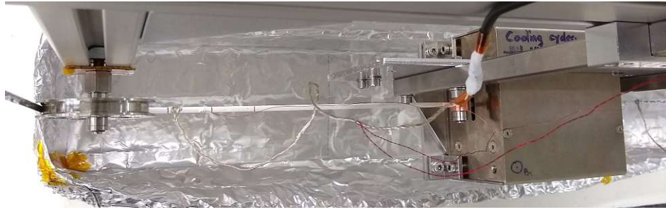
Figure 4.15 – Picture of the silver capped sample in the experimental setup. Sample and magnet were fully immersed in liquid nitrogen during the scan.
