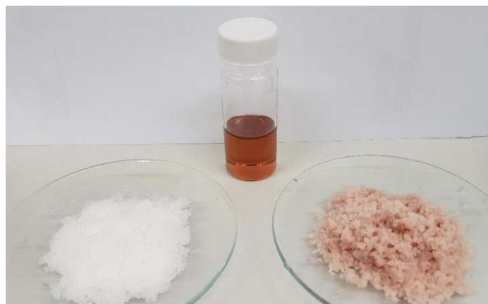
Figure 112. Starting materials choline Cl (front left), p -TsOH (front right) and the DES choline Cl/ p -TsOH (back).
