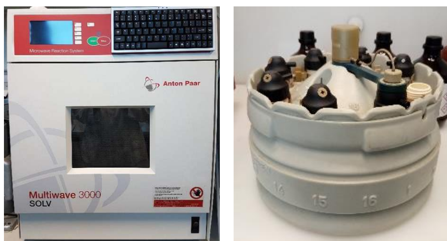
Figure 57. Microwave oven (left) and digestion unit (right) where car catalyst digestion was performed.
