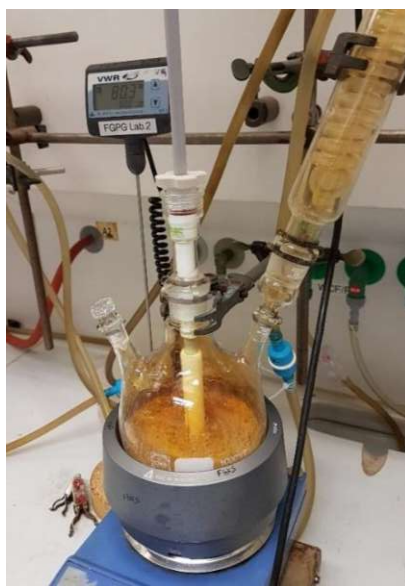
Figure 72. Upscaled leaching set-up on a 100 g catalyst scale.
