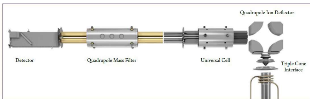
Figure 60. Simplified drawing of ICP-MS system with Universal cell technology.
