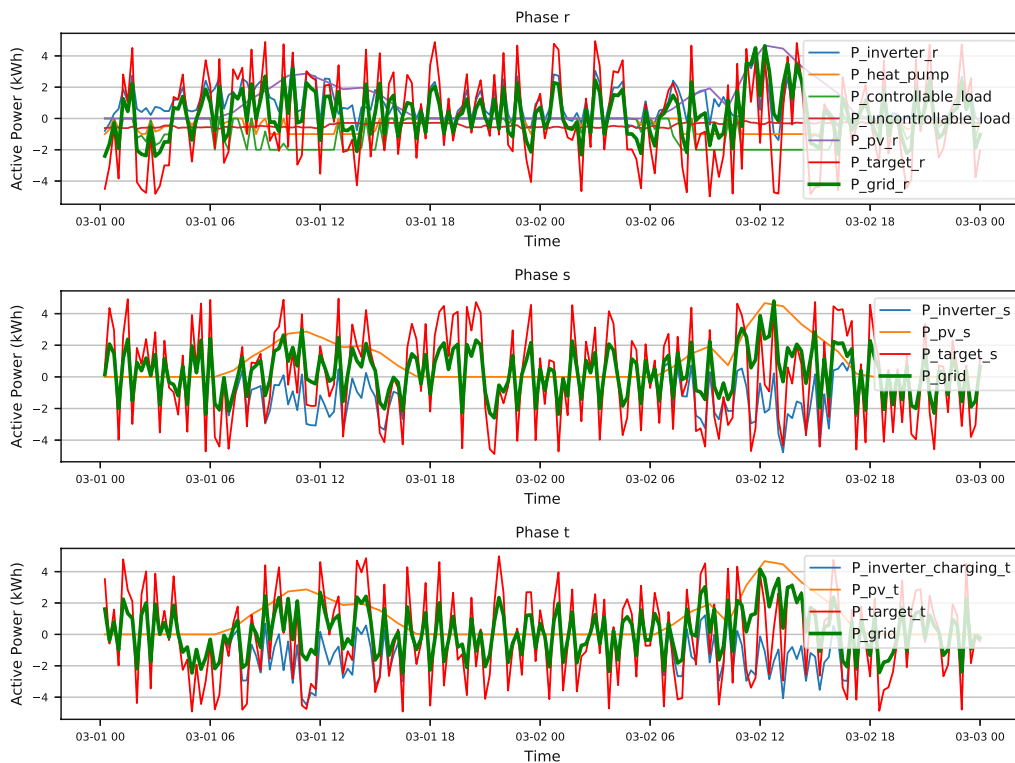
Figure 11. Per-phase active power controllable and disturbance variables for passive house and weight scenario (S, U, G) = (0, 0, 1)
