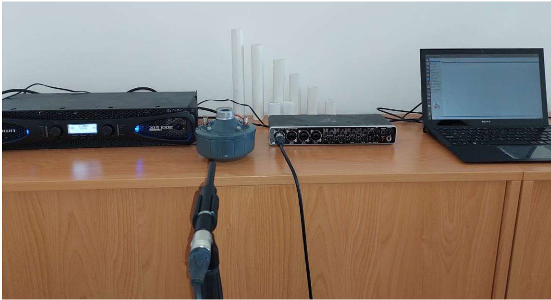
Figure 4.2: Used playback and recording devices. Front: Microphone. Back: The set of tubes with diameter 32 mm. Middle from left to right: Pre-amplifier, sound driver, microphone interface and laptop.
