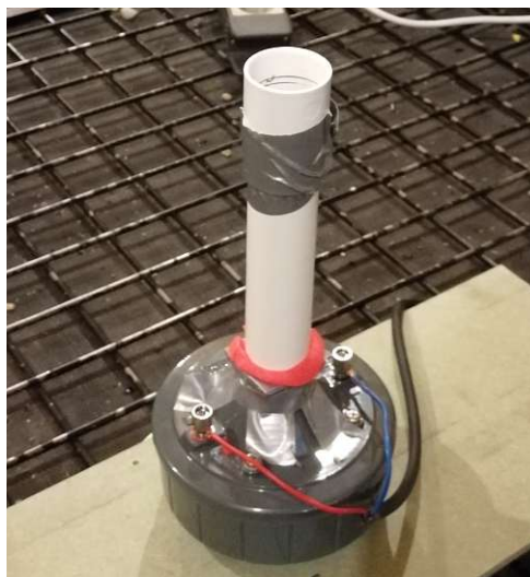
Figure 4.4: The tube placed on top of the driver and carton with the slit, isolated with play doh.
