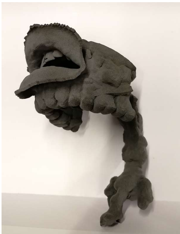
Figure 4.6: The 3D-printed vocal tract model, used in the final phase of the lab experiments.
