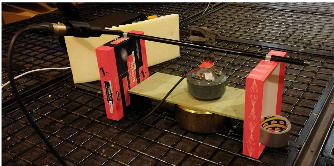
Figure 4.7: The set-up of the vocal tract model on top of the sound driver. The model was supported by a rod and placed at a distance of 30 cm from the microphone.
