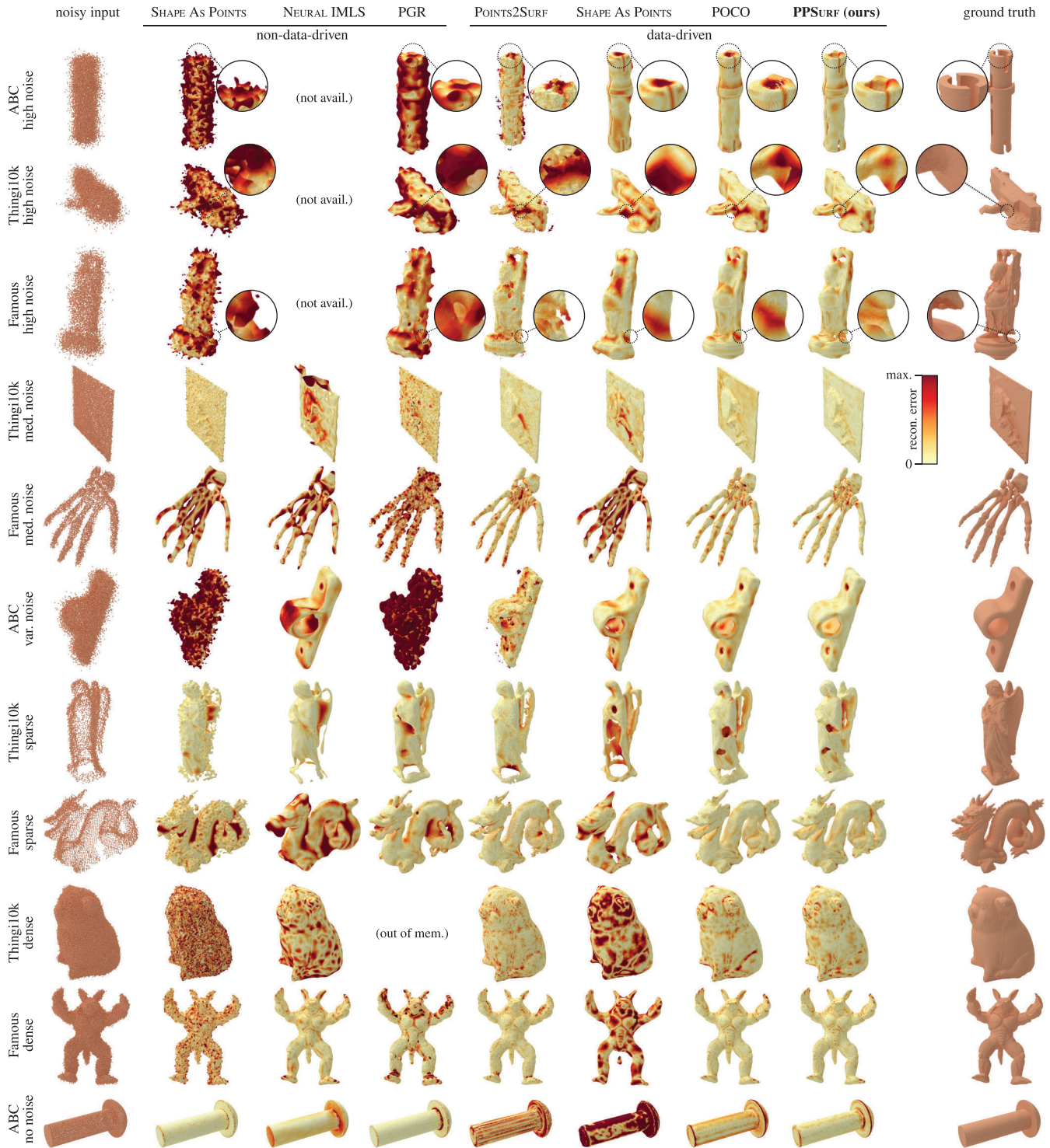
Figure 4: Qualitative comparison to all baselines. We evaluate one example from each dataset variant (except for the no-noise variants, where we only show one example due to space constraints). Colours show the distance of the reconstructed surface to the ground-truth surface. Due to our combined local and global branches, PPSURF reconstructs details more accurately than the baselines, especially in the presence of strong input noise. Note that results for Neural IMLS are not provided by the authors for the high-noise dataset variants. See the supplementary material for a qualitative comparison on all shapes in our test sets.
