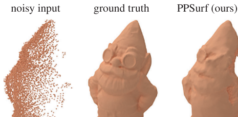
Figure 7: Limitations. Our method struggles with reconstructions of large missing areas in the input point cloud since we did not incorporate any generative model capabilities.
