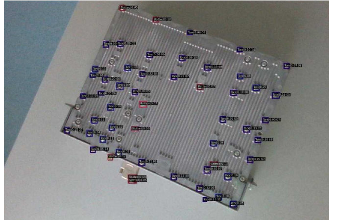
Fig. 5: Screw detection example Detections on a real validation image using FCOS. The blue bounding boxes show correctly detected and classified screws. Incorrect classifications are shown in red.
