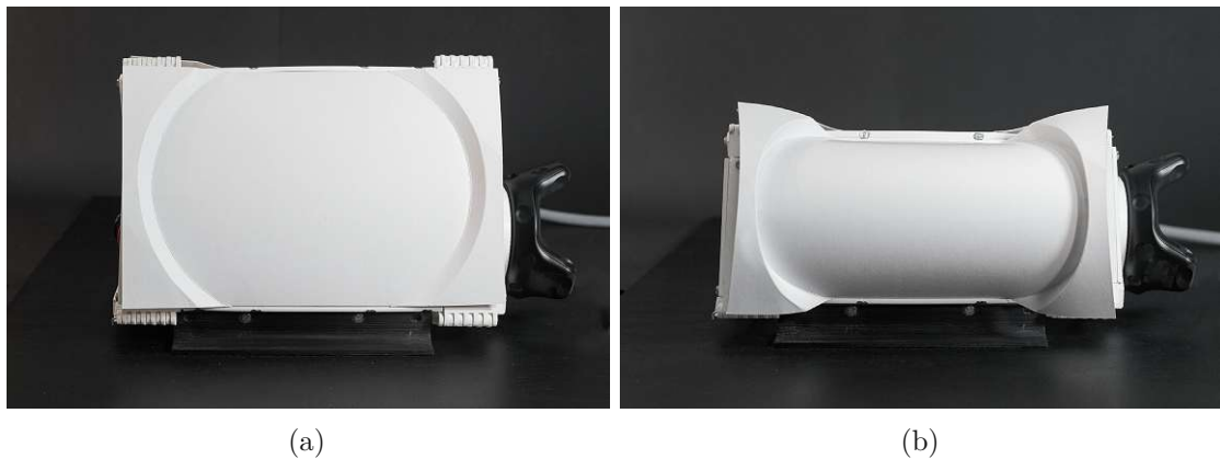
Figure 5.6: Shiftly mounted on the table and with an attached Vive tracker. In (a), the origami is extended, and in (b) the origami is contracted.
