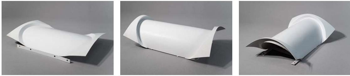
Figure 5.3: Fabricated origami structure
