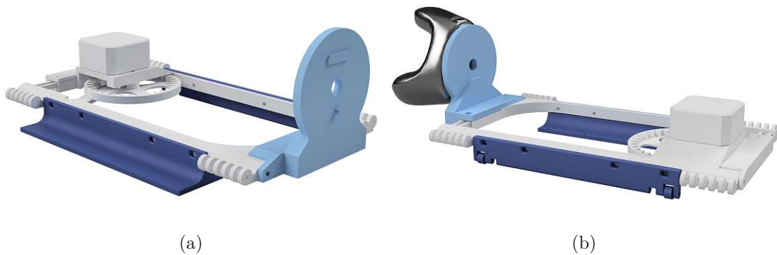
Figure 3.12: Frame with an attached stand and the VIVE tracker attachment. The stand is shown in dark blue, and the VIVE tracker attachment is rendered in light blue. (a) shows the front side with no VIVE tracker mounted, and (b) shows the back side with a tracker mounted.
