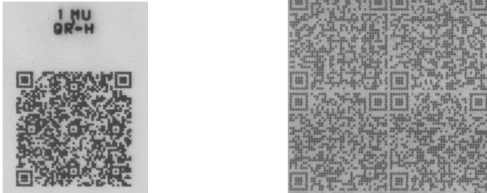
Figure 3.2: Microscope images with 100x magnification of a single QR-Code on the left and a matrix of QR-Codes on the right, ablated with 1 \mu\text{m} pixel size on a sample with 10 \text{ nm} CrN on a glass substrate.
