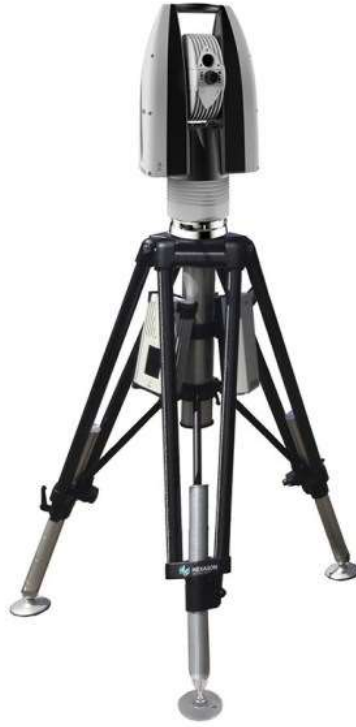
Figure 5.2 Leica Absolute Tracker AT960-MR (hexagon.com, n.d.)
