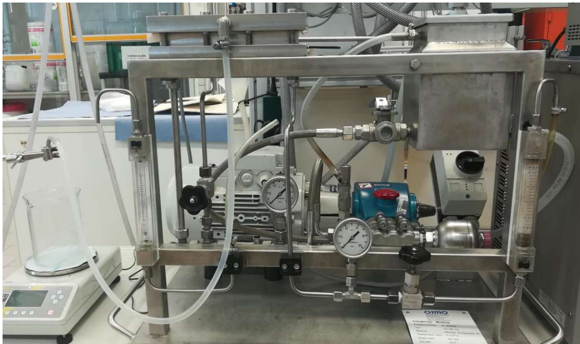
Figure 23. Membrane filtration unit.
