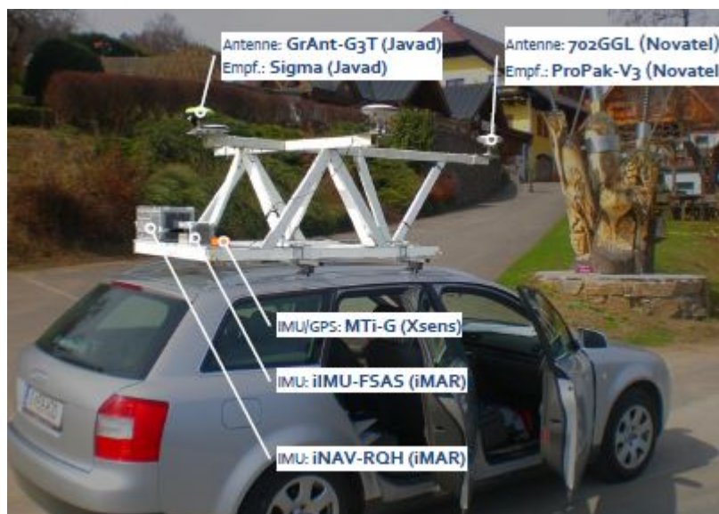
Figure 37: GNSS and IMU sensors mounted on the car's roof for a test drive of TU Graz in the past [Lae10]
