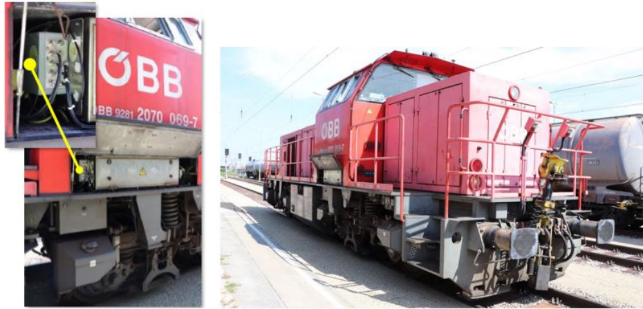
Figure 15: ÖBB tests of the inertial measurement system iRailLoc-C [iMa21]
