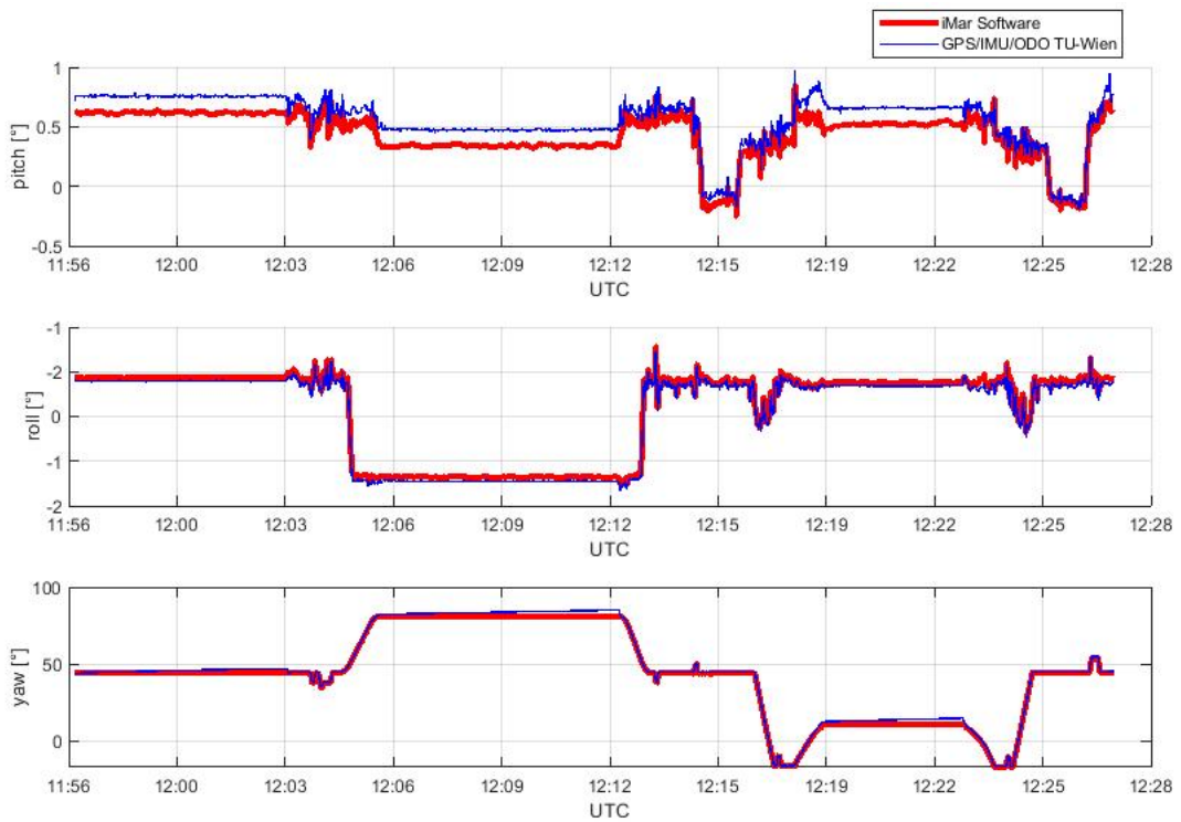
Figure 33: Roll/Pitch/Yaw solutions processed by TU-Wien Software and reference software
