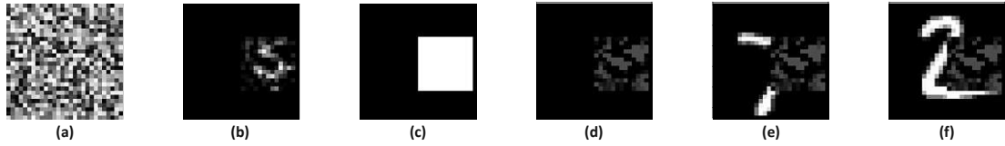
Figure 7.13: Process of trigger generation in the second Conv layer of the LeNet. (a) Initial input trigger. (b) Gradients of the selected neuron. (c) Mask created through gradients. (d) Final trigger after loop. (e) and (f) are two images with the applied trigger.
