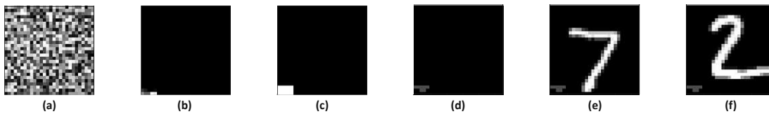
Figure 7.12: Process of trigger generation in the first Conv layer of the LeNet. (a) Initial input trigger. (b) Gradients of the selected neuron. (c) Mask created through gradients. (d) Final trigger after loop. (e) and (f) are two images with the applied trigger.
