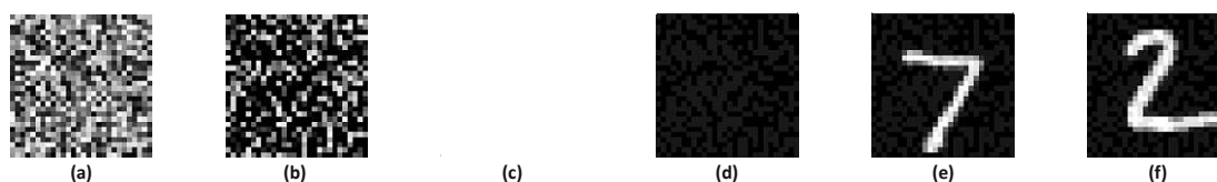
Figure 7.15: Process of trigger generation in the first layer of the MLP. (a) Initial input trigger. (b) Gradients of the selected neuron. (c) Mask created through gradients. (d) Final trigger after loop. (e) and (f) are two images with the applied trigger.
