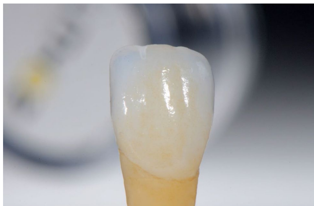
Figure 5. 3D-printed crown using a bi-material printing approach to combine pigment-containing lithium disilicate in the core with unpigmented lithium disilicate in the shell. Source: Lithoz GmbH.
