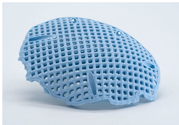
Figure 6. 3D-printed cranial implant made from hydroxyapatite. Source: Lithoz GmbH.
