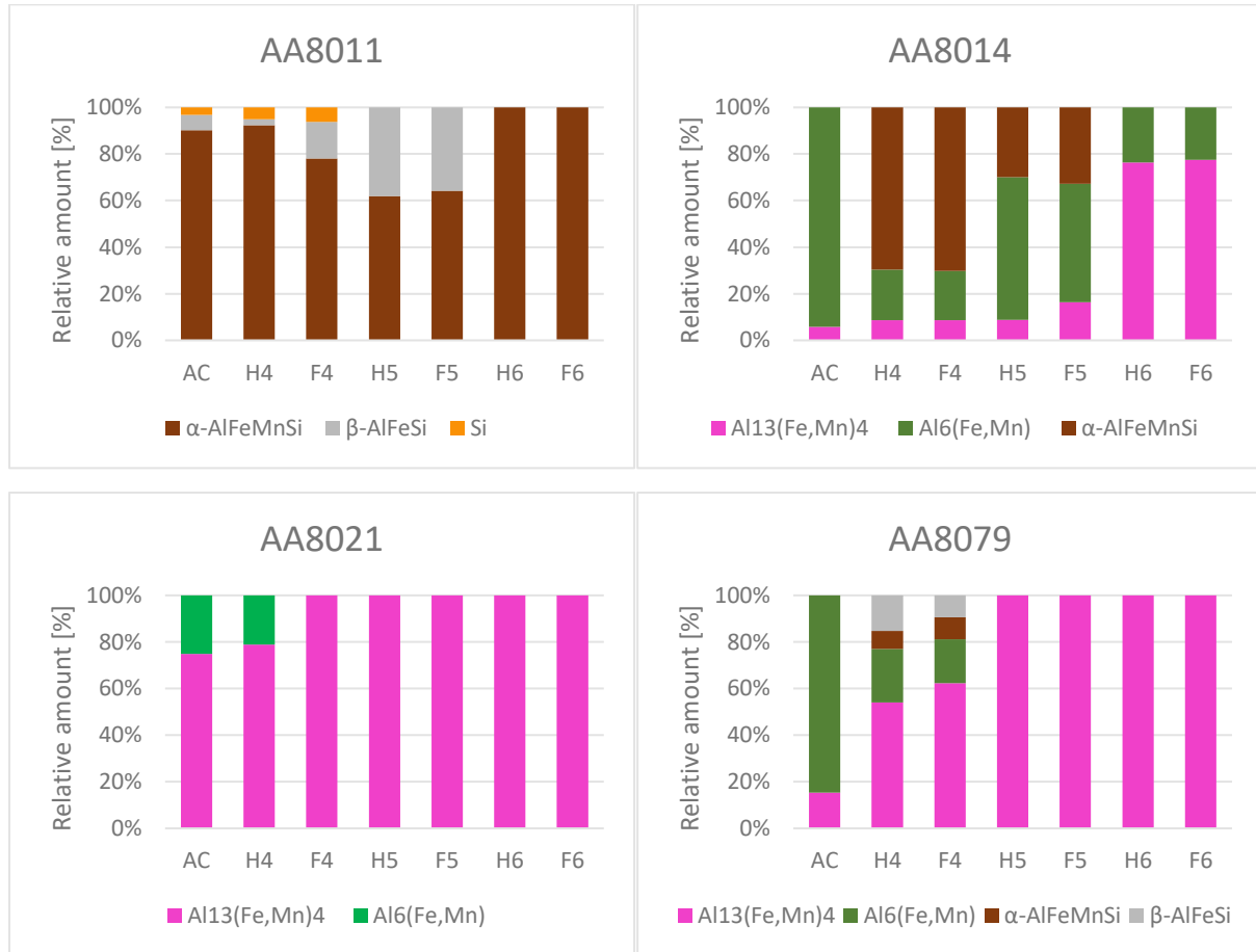
Figure 59: Results of the XRD analysis of the bulk samples (based on wt.%)
