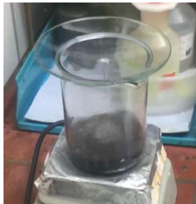
Figure 29: Dissolution of the aluminium matrix - boiling phenol with added Al sample
