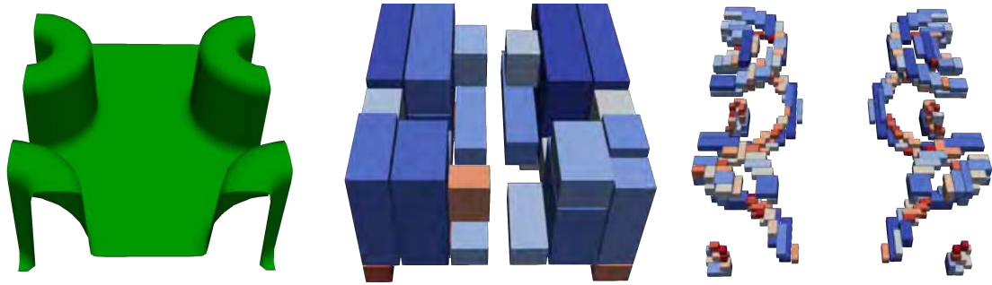
(a) Interface extracted from Level 0 . (b) Block placement on Level 1 . (c) Block placement on Level 2 .
