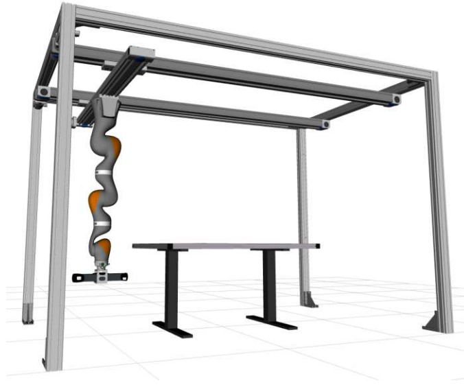
Figure 3.2: Visualization of the robotic system including the linear axes. It is defined by means of a URDF file to be used in MOVEIT.
