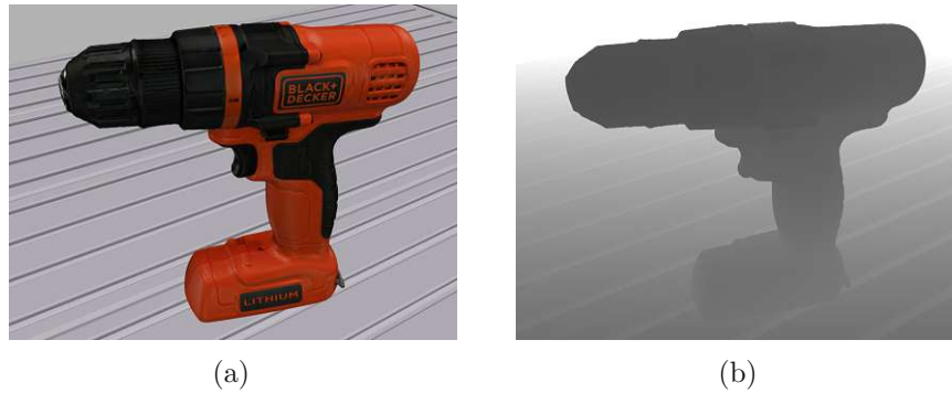
Figure 2.11: An RGBD image consists of (a) a color image and (b) depth information.
