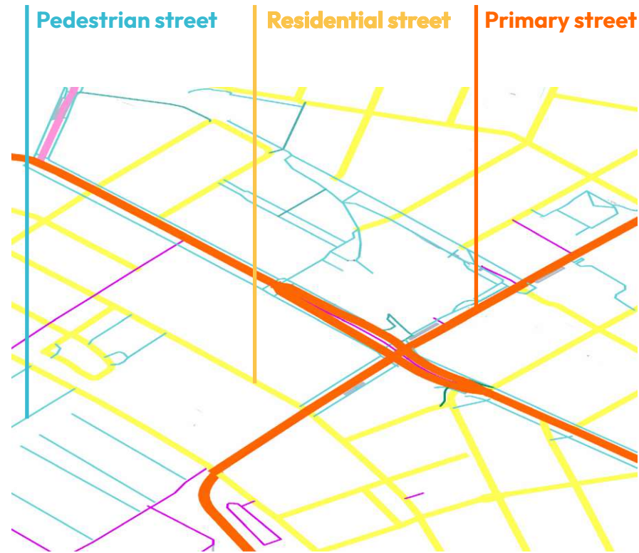
Figure 53: OSM Street Categories, exported from FME in meshes of different widths and highlighted in Unity by category
