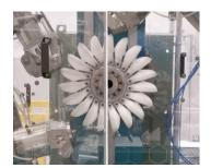
Fig. 1: Left: Test setup in the hydraulic laboratory of IET. Right: Isosurface of water coloured by the normalized flow velocity for one time step. The AR app visualizes the time series of the transient calculation results and provides the user a 3D view of the AR object, that can be zoomed and rotated.
