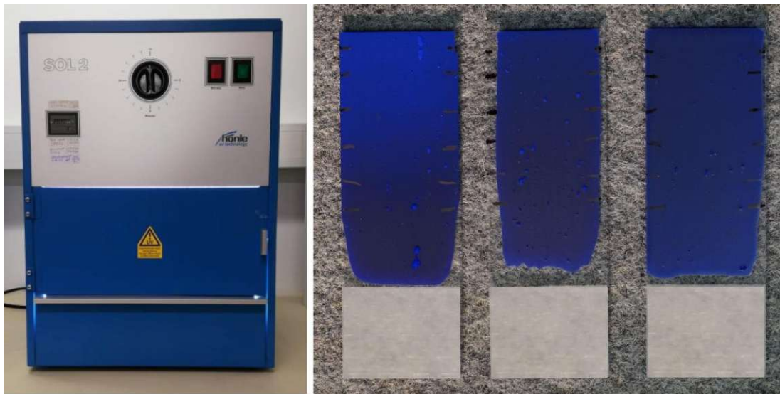
Fig. 12: UV-light aging chamber used and representative set of samples aged.
