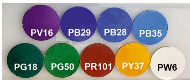
Fig. 1 Set of 9 pure pigment powder pellets analyzed by LIBS
