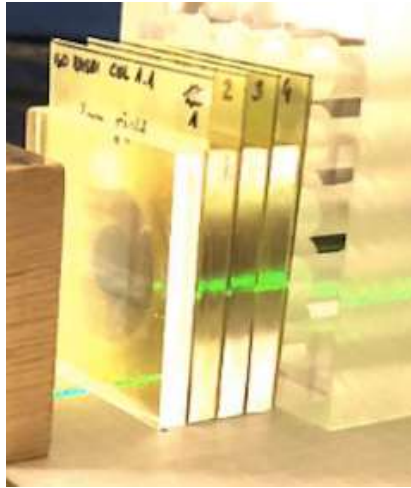
Figure 2-4: EBT3 films inserted at different depths of the phantom
