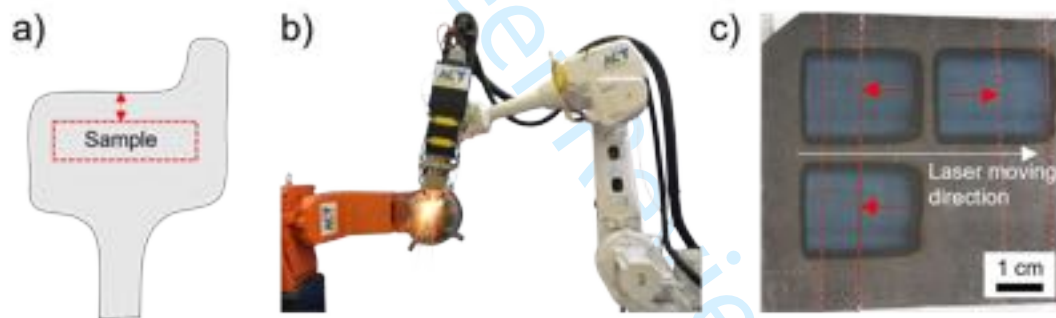
Figure 1: (a) The samples for the laser treatment are cut out from wheels ~1 cm below the tread surface followed by uniform heat treatment. (b) shows the laser system which is used for applying thermal loads. (c) gives an exemplary wheel plate sample after three laser surface treatments are conducted. Red dotted lines and arrows show the cross-sectional cuts which are analysed by light optical microscopy.
