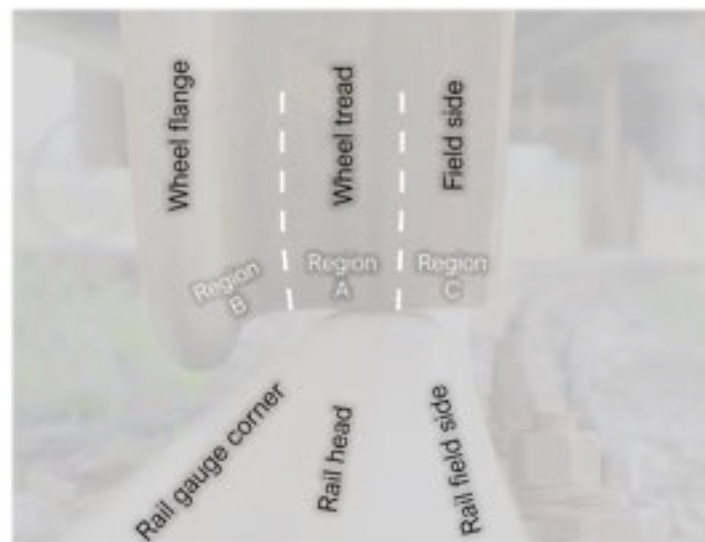
Figure 2: Different possible regions of the wheel-rail contact (image adapted from [59])
