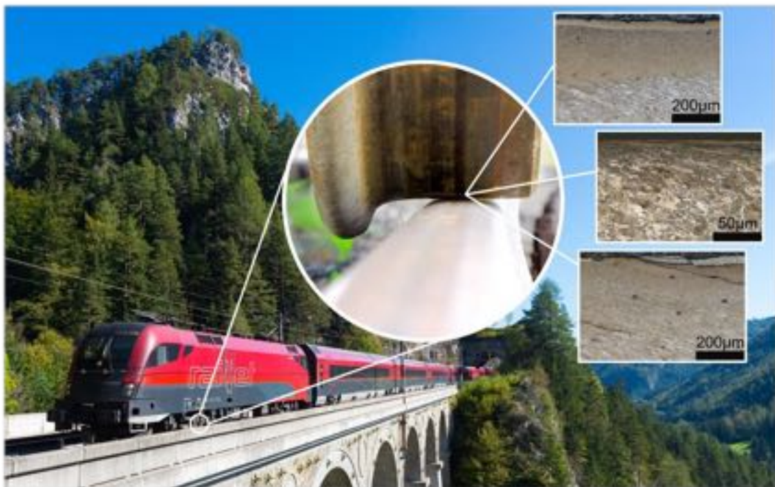
Figure 1: Several tons of wheel load and an open system tribology within \sim 1 \text{ cm}^2 of contact zone, the outstanding complexity of the wheel-rail contact results in a wide variety of evolving near-surface microstructures during service. [58], [59]
