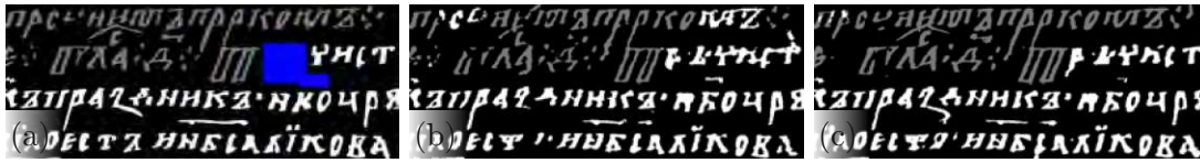
Figure 4.42: Segmentation results. (a) Ground truth image. Blue regions are ambiguous regions that are excluded from the numerical evaluation. (b) Result gained on the white light channel. (c) Result achieved on all spectral ranges.
