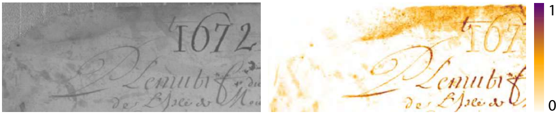
Figure 4.1: ACE based target detection. (Left) Manuscript imaged at 500 nm. (Right) ACE result. The result is color coded as indicated by the bar on the right.
