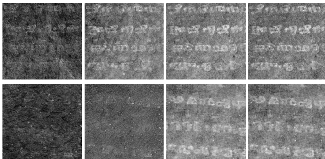
Figure 3.13: Enhancement results. From left to right: UV reflectography image. PCA image. Coarse enhancement result. Fine enhancement result.
