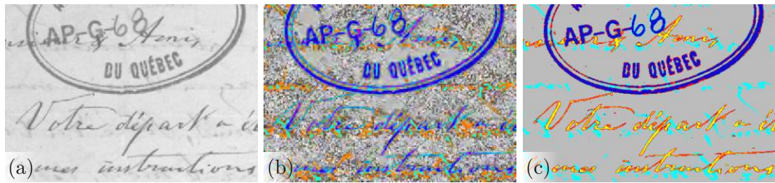
Figure 4.10: Clustering of multispectral image. (a) Image acquired at 500 nm. (b) k-means output. (c) GMM output.
