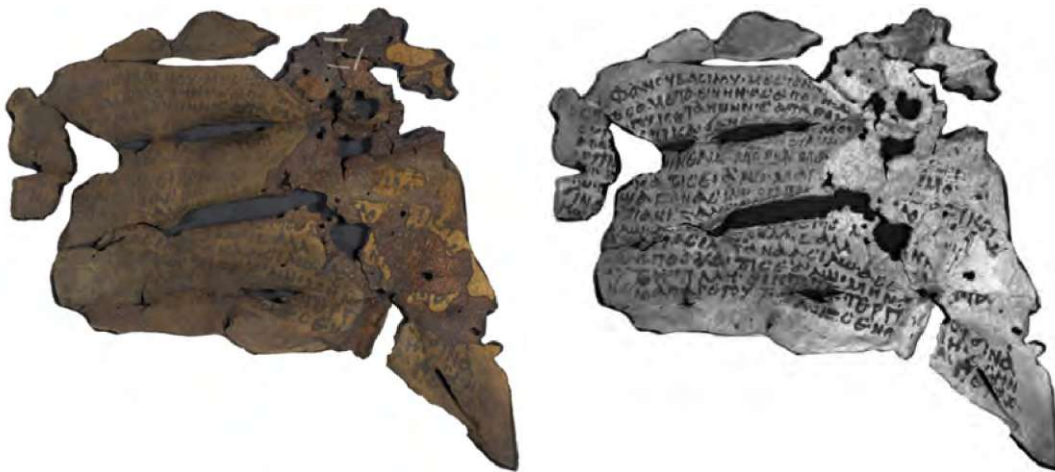
Figure 3.8: Fragment with the id SR22 A560, found in Egypt. (Left) Image taken under white light. (Right) NIR reflectography image (870 nm).
