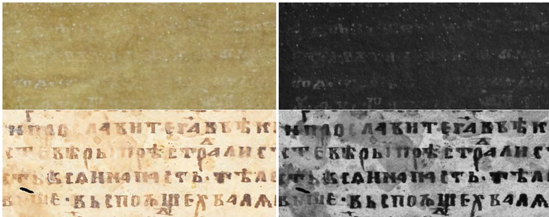
Figure 1.3: Exemplar input images used for enhancement (top row) and binarization (bottom row). White light images are shown on the left and UV images on the right.
