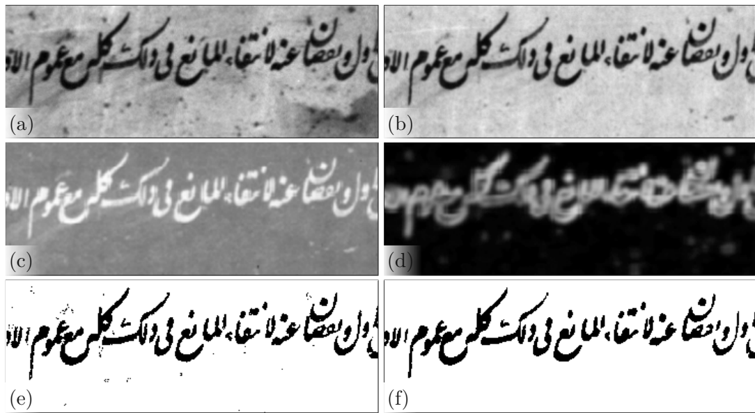
Figure 2.11: Binarization output by Hedjam and Cheriet [HC11b]. (a) Multispectral channel in the visible range. (b) Multispectral channel in the NIR range. (c) Pattern persistence image. (d) Pattern energy image. (e) ML result using reflectance values. (f) Result.
