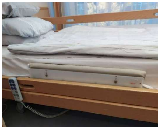
Fig. 2: The sensor-bar to detect the residents' movement if they get out of the bed.
