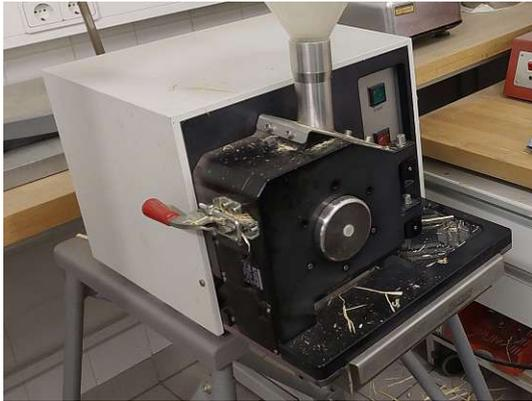
Fig. 15.: *Closed cutting mill*
