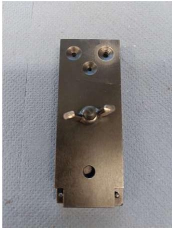
Fig. 22.: *Closed mould*
