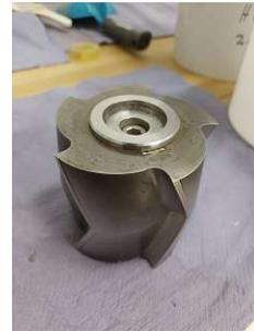
Fig. 18.: *Rotating knife within the cutting mill*
