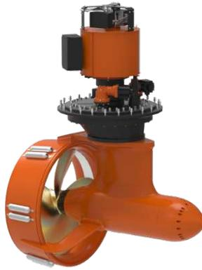
Figure 4: Azimuthing podded propulsion drive.
