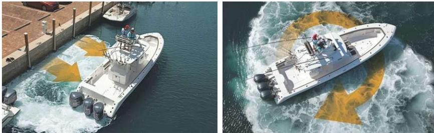
Figure 1: Yamaha Helm Master commercial images showing facilitation of a lateral unmooring maneuver (left) and a stationary rotation maneuver (right) by adjusting the outboard motor operating angles and thrusts automatically.
