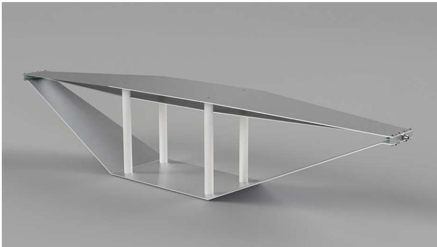
Fig. A.1: Picture of the developed asymmetric TEM cell from [20].
