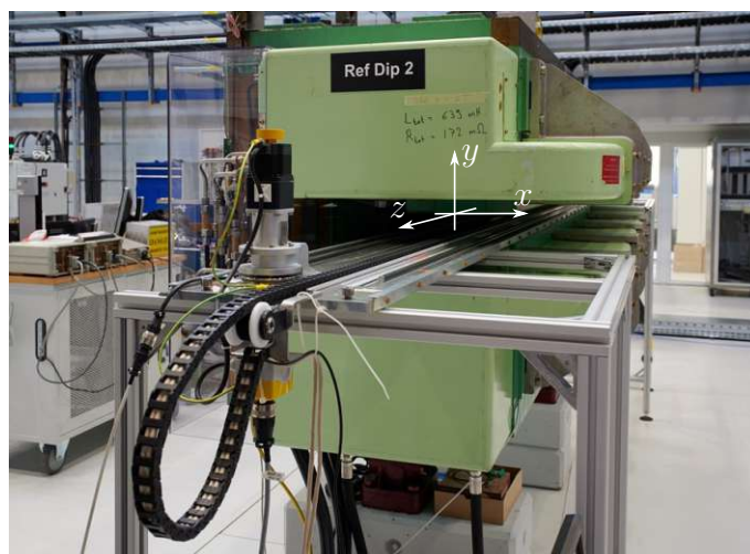
Figure 4.1: For the metrological characterization campaign the translating fluxmeter is installed in the reference dipole. The orientation of the coordinate system used in this work is shown here. For the location of the origin refer to text and Fig. 4.2.
