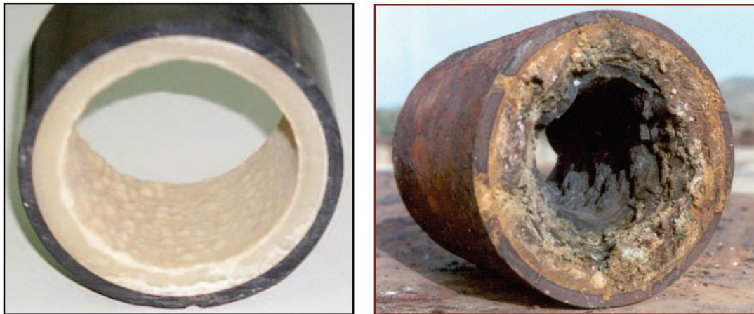
Figure 6.9: Scaled geothermal pipes (left: calcite, right: mixture of \text{SiO}_2 and sulfide) (Andritsos et al. 2014)
