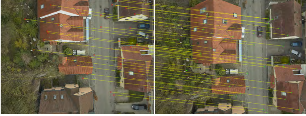
Figure 3.18: Example of IMG-to-IMG matches. Here, only every 500-th correspondences is shown of the 16377 correspondences that have been found in total. This image pair is taken from the example in section 4.4.
