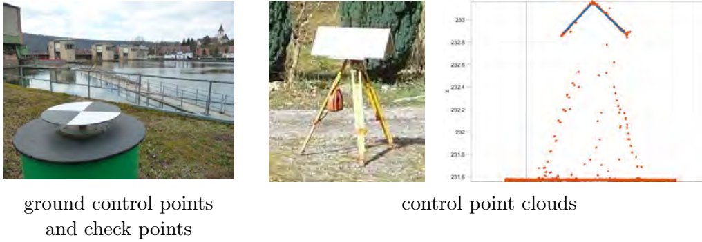
Figure 4.17: Ground-truth-data for images and lidar. On the right, the alignment of the lidar points (orange) and the control point cloud (blue) is shown after the hybrid adjustment.
