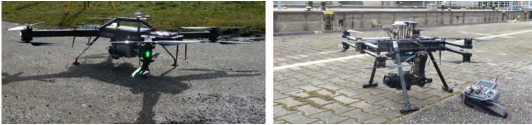
Figure 4.18: UAVs used for data capturing. Left: Riegl RiCopter with VUX-1LR scanner and two Sony Alpha 6000 cameras. Right: CopterSystems CS-SQ8 copter with PhaseOne iXU-RS 1000 camera.
