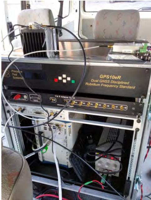
(a) DIST measurement campaign, TX setup of hardware in the van.
