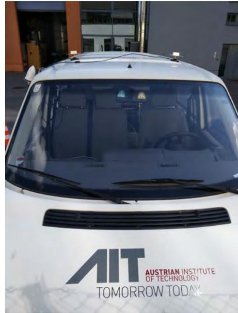
(b) DIST measurement campaign, TX and GNSS antennas on vans roof.
