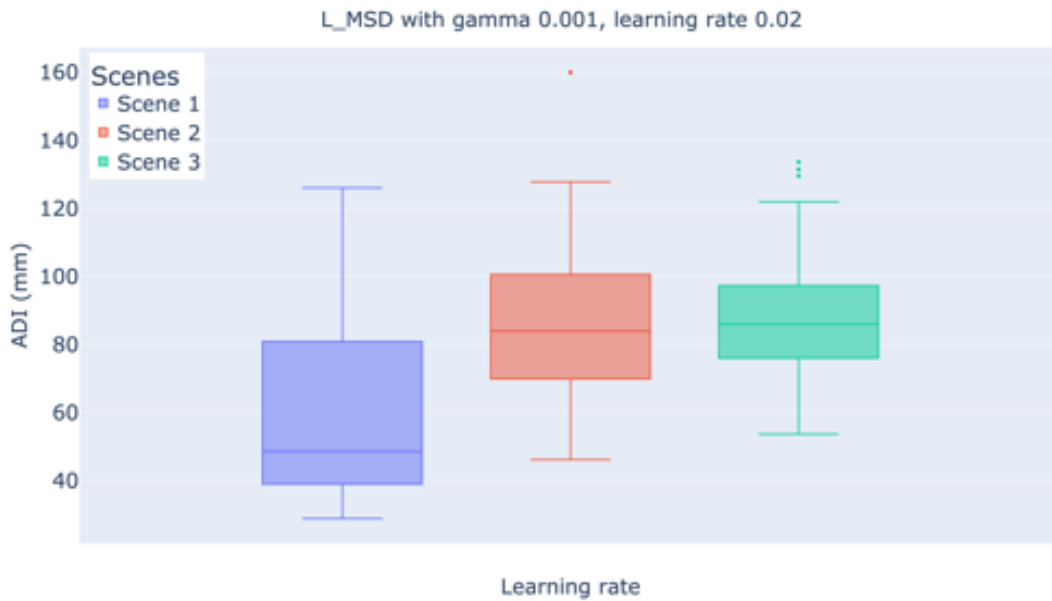
Figure 5.27: The ADI result of heuristic initialization of the pipeline over three different scenes.
