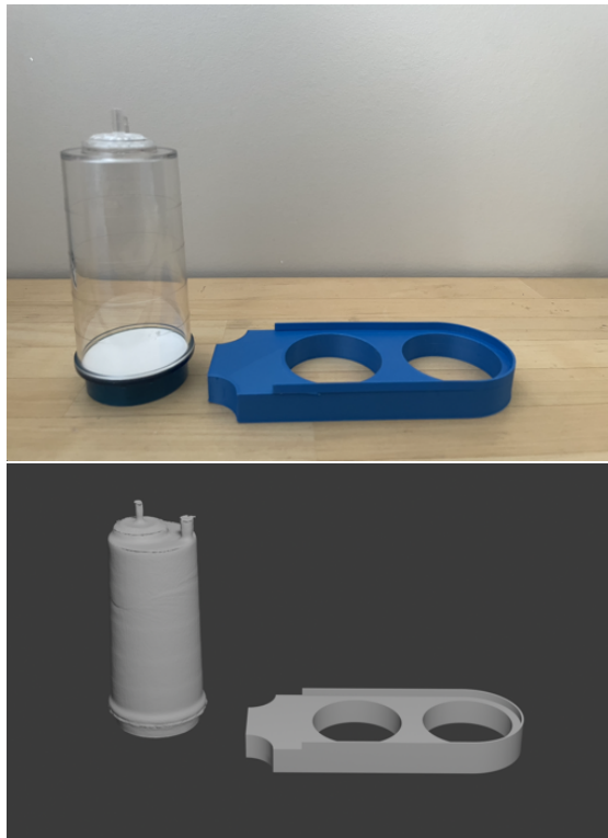
Figure 4.1: Objects included in the Tracebot dataset. On the top, we show authentic images of the mentioned objects. From left to right, there is a canister and drain tray. On the bottom, we show the rendered CAD models for each object.
