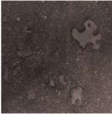
Figure 41: Bed material AC2 after trial with particle agglomerates that formed atop the distributor plate
