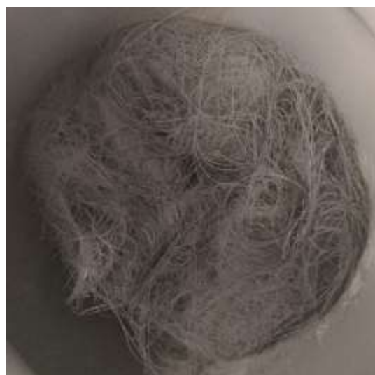
Figure 59: Fine powder of carbon and bed material on the filter
