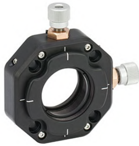
Figure 2.19.: XY Translation mount CXY1A from Thorlabs used to mount all 1" optics
