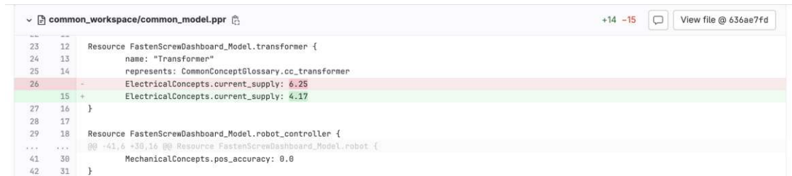
Figure 6.28: Model-based merge with the inheritance of values into the common model from the domain-specific model (electrical) performed by the CIA Bot .
