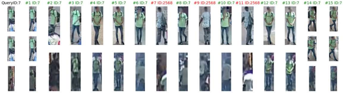
Figure 4.2: Proposed Multi-View Retrieval Results. Since we are working with calibrated multi-camera setup, one object can be seen from from multiple views, thereby enhancing the results. In this figure a query is seen from 3 different views. First retrieved result is seen from 3 different views, whereas the second result is seen from 2 different views. False positives are shown in red.
