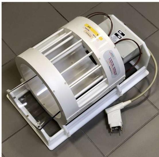
**Figure 3.4:**  $^2\text{H}/^1\text{H}$  dual-tuned quadrature bird-cage head coil used for phantom and in vivo relaxation time experiments.
