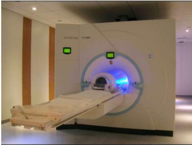
**Figure 3.3:** Experimental 7T whole-body MR scanner from Siemens, located at the Highfield MR Center. Figure taken from [62].
