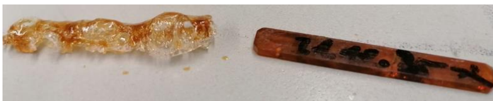
Figure 21: Comparison of a formulation containing 50 mol% DI-C cured via cROP (left) and aROP conditions (right). Both specimens show colouration due to relatively long exposure times (600 s) and high post-curing temperatures (120 °C). The cROP specimen is highly porous due to decarboxylation reaction, while the aROP specimen does not show porosity.
