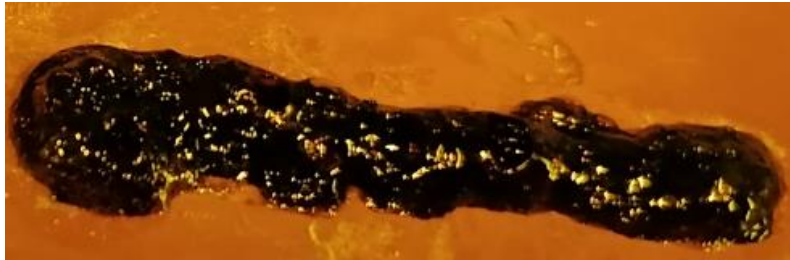
Figure 8: Bulk curing test with Et-C at 100 mW cm -2 light intensity. Due to the high light intensity, the formulation is strongly darkened and porous through a decarboxylation side reaction.
