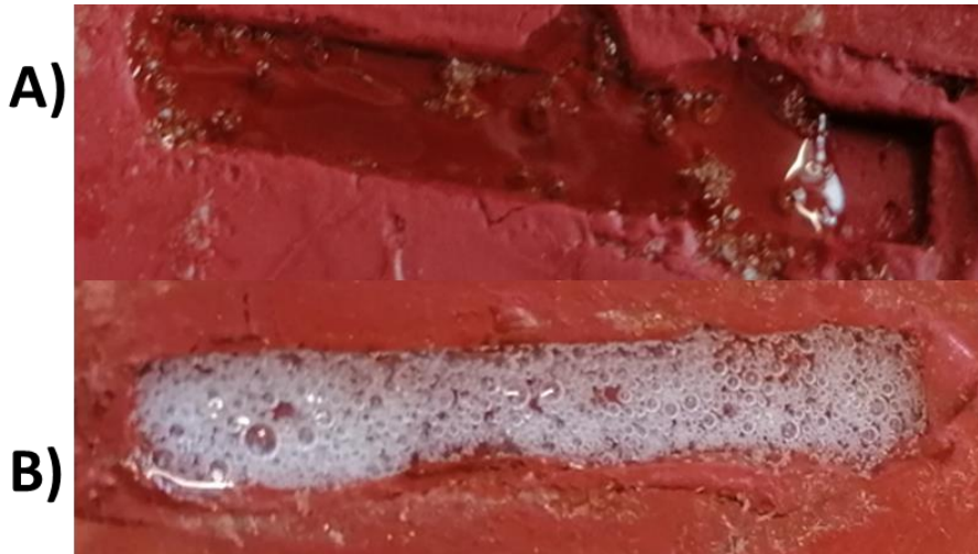
Figure 9: Comparison of the formulation after irradiation and before post-curing (A, low bubble formation) and after 60 min post-curing at 50 °C (B, strong bubble formation)
