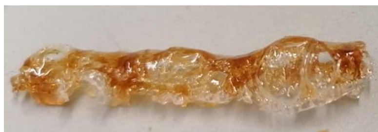
Figure 7: Bulk cured sample from Ar-C under cROP conditions, using 1 mol% S-Sb as initiator and 25 mol% DI-C. The samples showed clear signs of decarboxylation, which causes highly porous structures.
