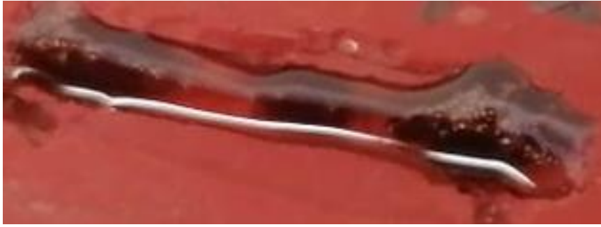
Figure 11: Inhomogeneities of the formulation using IC 290 observable as dark spots within the formulation after irradiation
