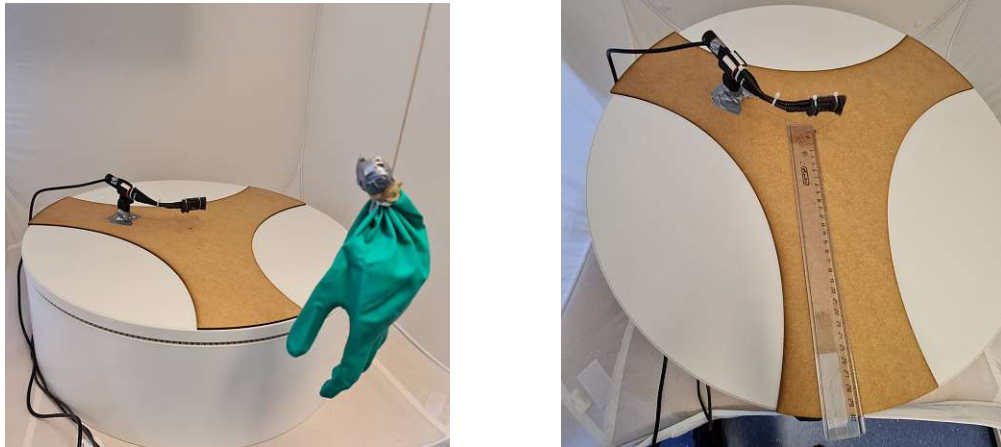
(a) Turntable with the "Hand"-Pendulum. (b) Turntable with a ruler to mark the distance.
