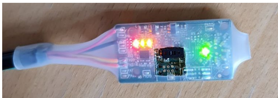
Figure 1.1: The sensor used, an STMicroelectronics VL53L1X (black element at the centre of the board), with the gyro sensor connected to the green LEDs to the right to visualise the pose of the sensor.
