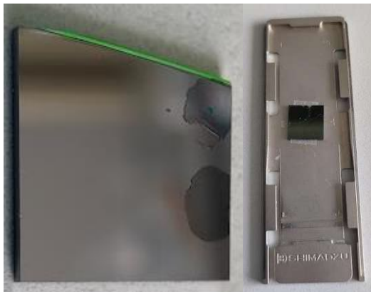
Figure 7: (Left) Pristine Si-Wafer without a polymer film and (right) a sample holder used for the Si-wafer to transfer the sample to the ion source of the MALDI-linTOF instrument.
