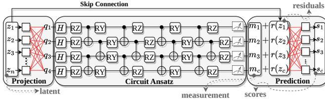
Fig. 8. Hybrid QNN with Four Qubits and Layers
