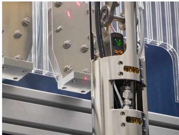
Abb. 5.4: Measuring the difference between the machine's and the part's coordinate system. The laser distance sensor in the lance also displays the measured distance, allowing for a correction. To achieve this, points in the point recipe are selected, carefully navigated to and the value on the display is read. Note, that the distance measured is lower than the minimum safety distance. This is explained in Figure 5.5. The other laser points in the image show the orientation of the CO2 jet nozzle.
