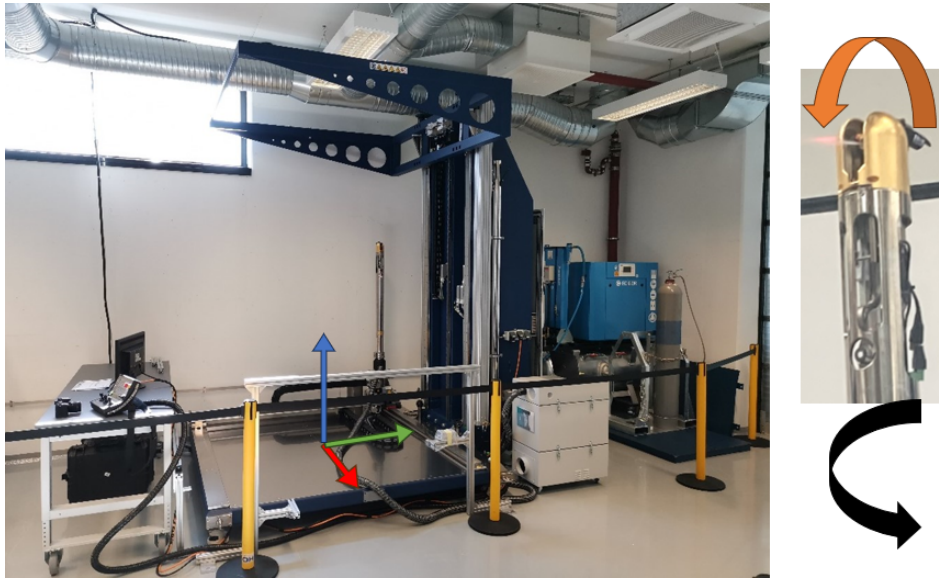
Abb. 3.2: Available degrees of freedom of the cleaning apparatus. The machine's cartesian coordinate system sits centered on the base plate with respect to x (red) and y (green). The origin of the z coordinate sits on top of the camera of the lance and thus not as depicted here. The coloring is the same as the coordinate system used by Open3D. The rotational degrees of freedom of the lance are the C (black) and R (orange) angles. Also visible in this image are the smaller lance and the laser pointers in the lance head which help orienting the CO 2 jet.
