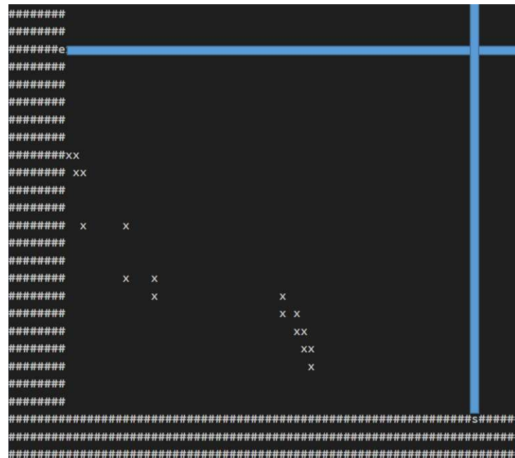
Abb. 4.8: Visualisation of the pathing using the pathing library. # are obstacles, s and e depict the start and endpoints. x depict corner points. The blue lines show where the 'highways' with lower weights are running along. As can be seen, the unmodified version creates many corner points which prolong cleaning operations since the lance has to turn in the direction where it is moving.
