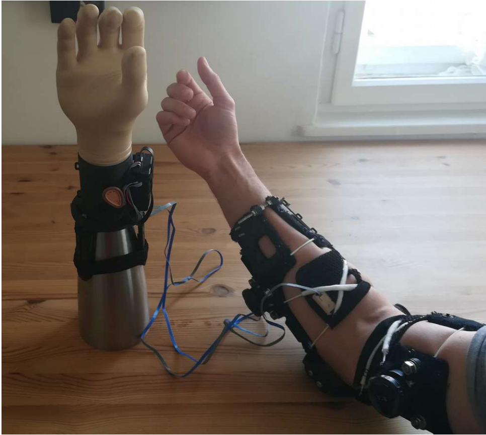
Figure 41: Test setup for people without an amputation. The rails are disconnected from the radial part, the quick disconnect adapter and the prosthetic hand are removed. The participant is able to don and doff the prosthesis and control the prosthetic hand with the help of the electrodes
