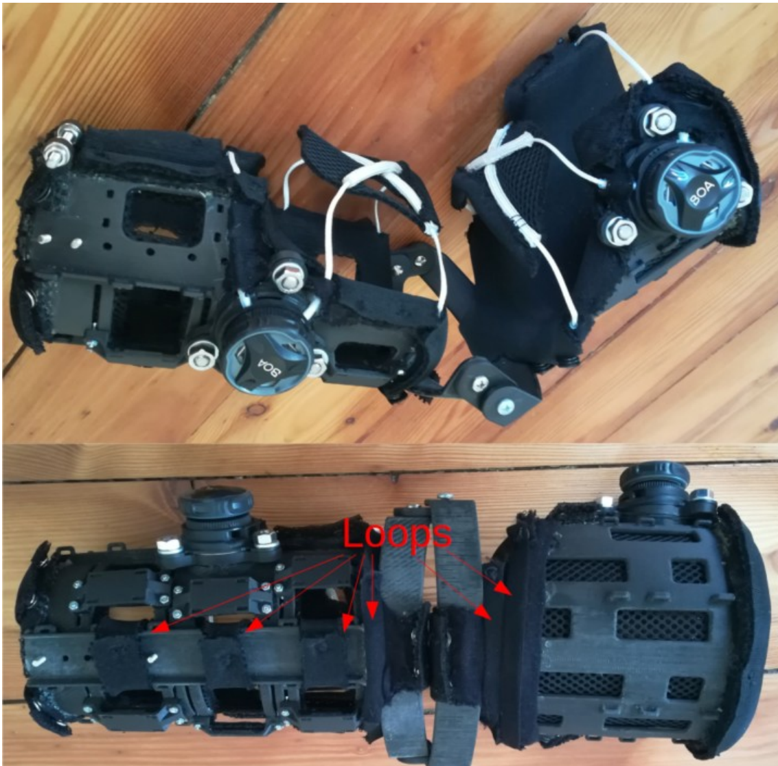
Figure 50: radial and humeral part of the BeneFit socket with second cushioning layer attached: above: seen from the side; below: seen from the back
