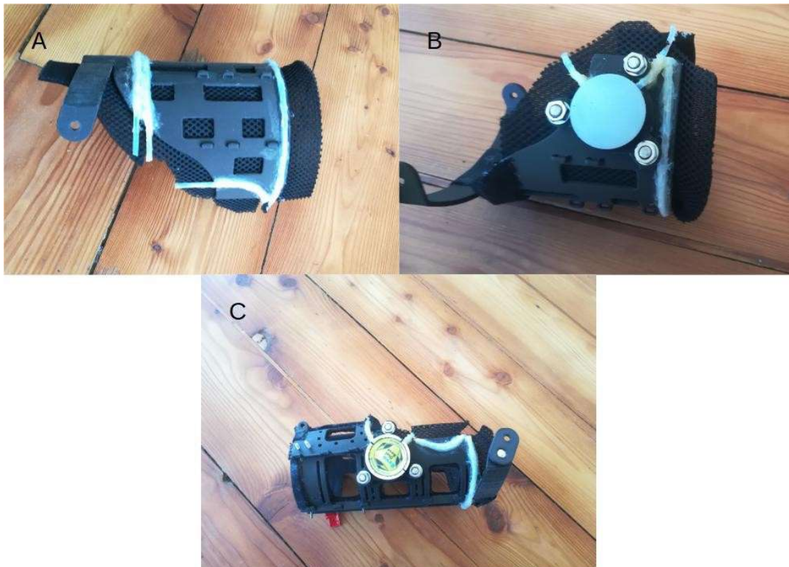
Figure 33: hard shell with cushioning material on the inside and tubing/ RevoFit2™ Lamination Dummy/RevoFit2™ Diagnostic Reel Base attached to the outside; A: right side humeral part; B: left side humeral part with RevoFit2™ Lamination Dummy; C: left side radial part with RevoFit2™ Diagnostic Reel Base
