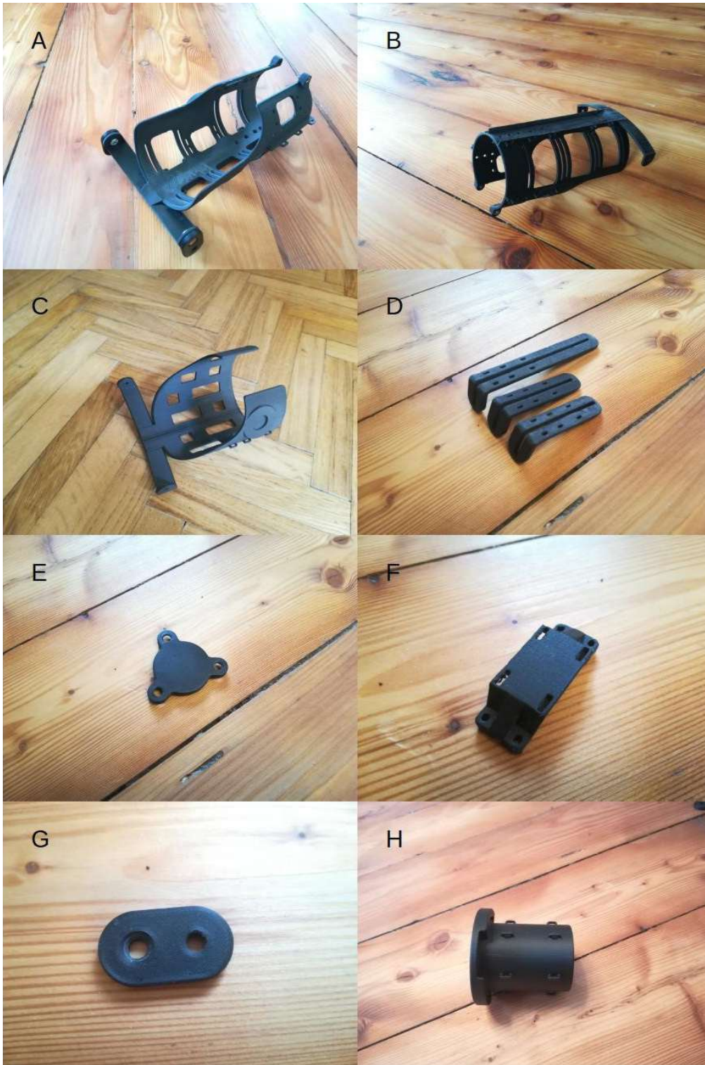
Figure 28: printed and post-processed parts: A: radial part from above (plates of double hinge joint attached); B: radial part from below; C: humeral part; D: rails; E: BOA installation disk; F: bridge; G: plate of double hinge joint; H: quick disconnect adapter
