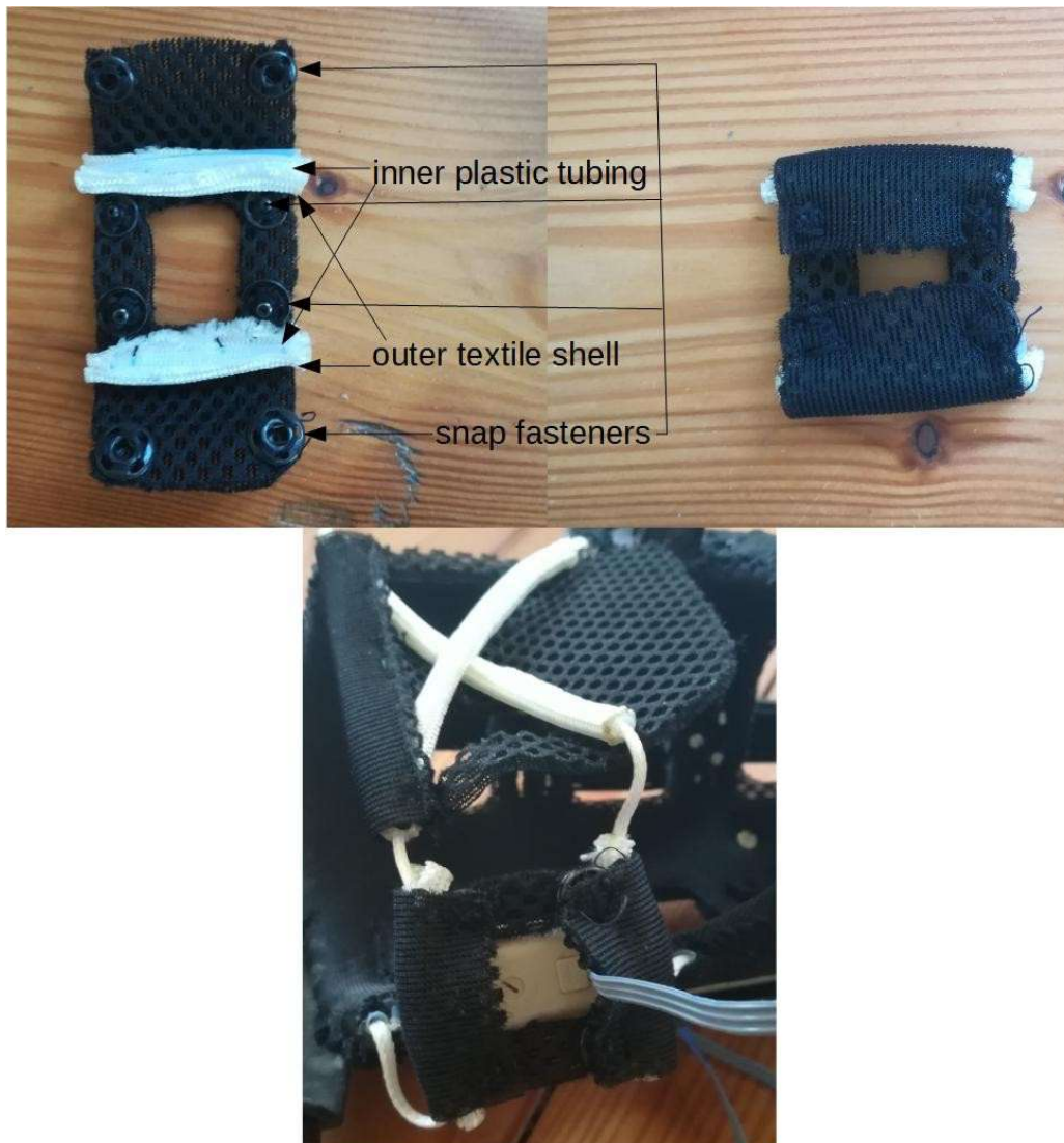
Figure 53: additional pad for fixation of an electrode, above on the left: open, inner plastic tubing, outer textile shell and snap fasteners are visible; above on the right: closed; below: mounted on laces with electrode attached
