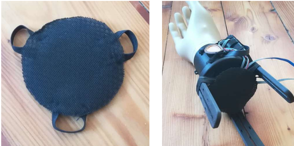
Figure 30: left: cushioning pad with 3 elastic bands attached; right: mounted cushioning pad to cushion the distal end of rail and quick-disconnect adapter.
