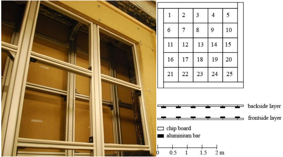
Figure 34. View (left) and schematic illustration (right) of the experimental modular double wall.
