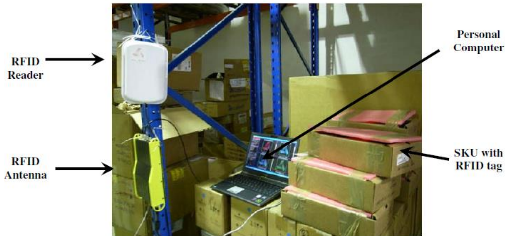
Figure 159: RFID technology implementation in warehouse environment for R-LRMS
