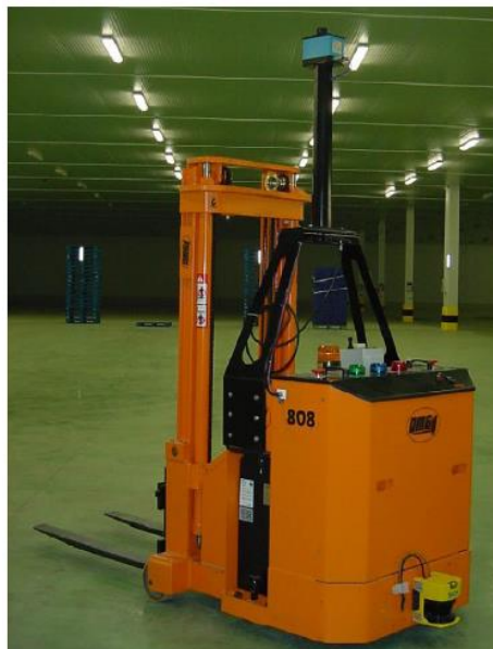
Figure 174: Modified OMG 808 FS fork-lift truck
