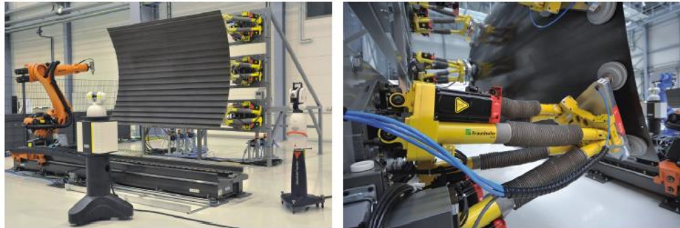
Figure 181: Prototype for Flexible Automated Holding Fixtures (FAHF). Fraunhofer IFAM
