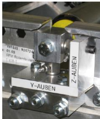
Figure 81: Roller Conveyor - Measurement Roller
