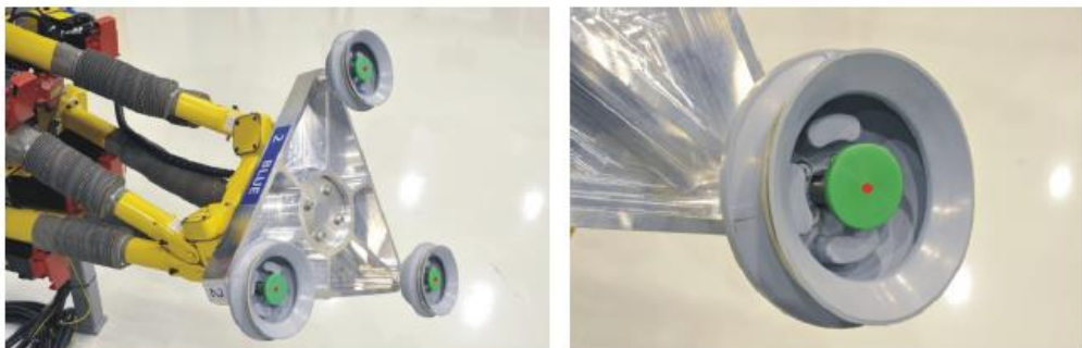
Figure 182: Gripper of the flexible automated holding figure. Fraunhofer IFAM
