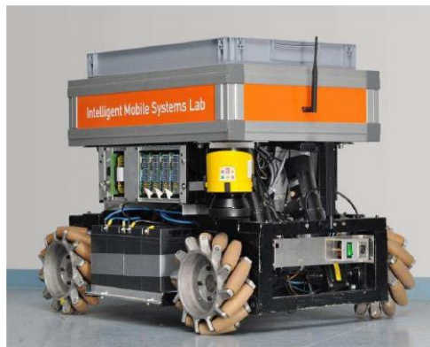
Figure 167: Sensor equipped omnidirectional transport robot
