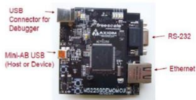
Figure 131: Freescale microcontroller board with embedded webserver and gateway
