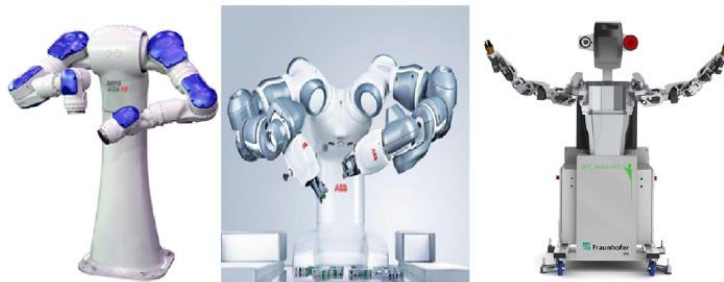
Figure 178: Dual-arm robot examples. Left to right YuMi (ABB), SDA 10F (Motoman/Yaskawa), Workerbot (pi4/Fraunhofer IPK)
