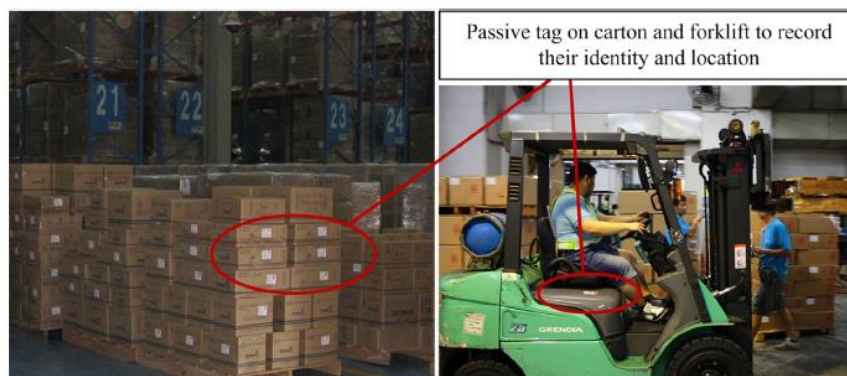
Figure 84: Passive RFID tags stuck onto cartons and forklift
