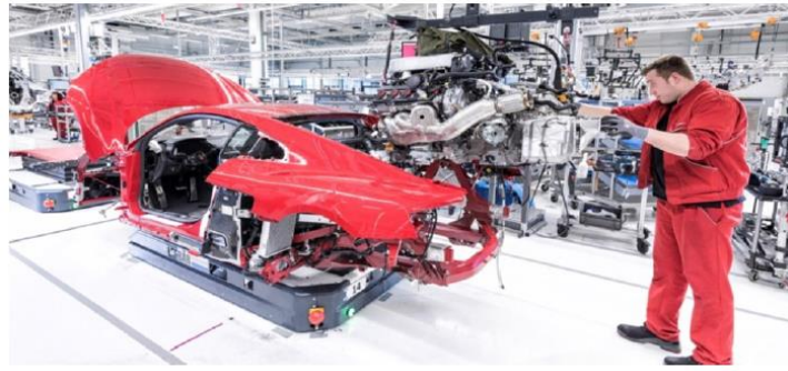
Figure 179: Mobile AGV robots for final car assembly (Krüger et al., 2017)
