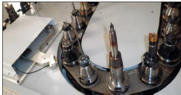
Figure 154: Tools with RFID tags on the machine rack (Dovere et al., 2015)
