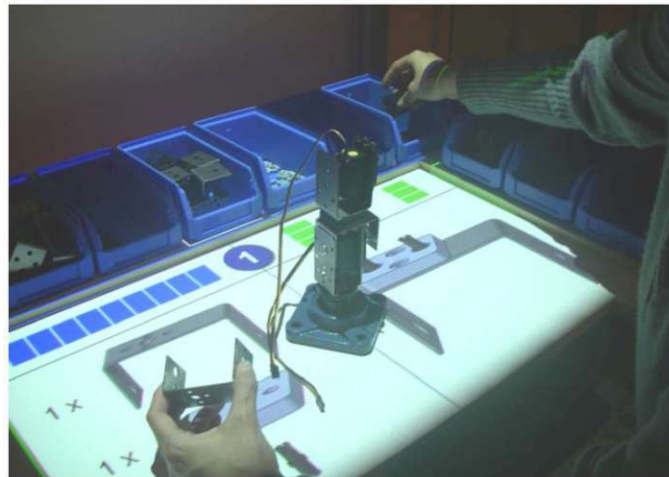
Figure 120: Projector-based assembly station
