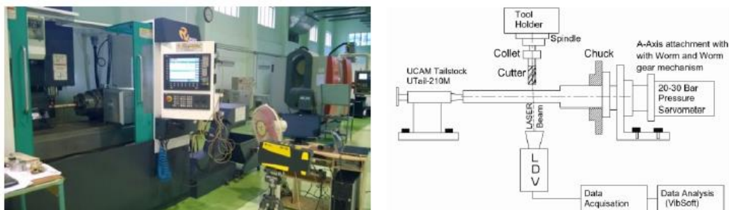
Figure 16: Online capturing of Acousto-optic Emissions - Experimental setup
