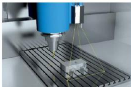
Figure 91: Camera-based monitoring system. From Heidenhain.
