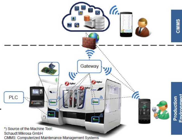
Figure 100: Decentralized data analysis using smart sensor network
