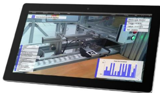
Figure 124: Process data visualization on a tablet PC
