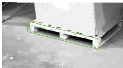
Figure 172: Pallet detection on full resolution
