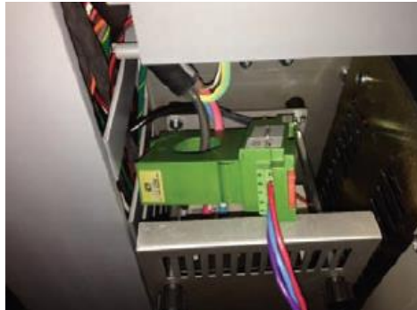
Figure 26: Hall effect current sensor
