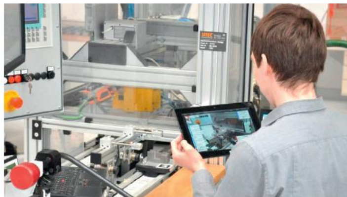
Figure 155: Augmented Reality monitoring example with marker-based tracking
