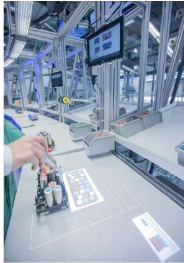
Figure 118: Worker information system for battery module assembly
