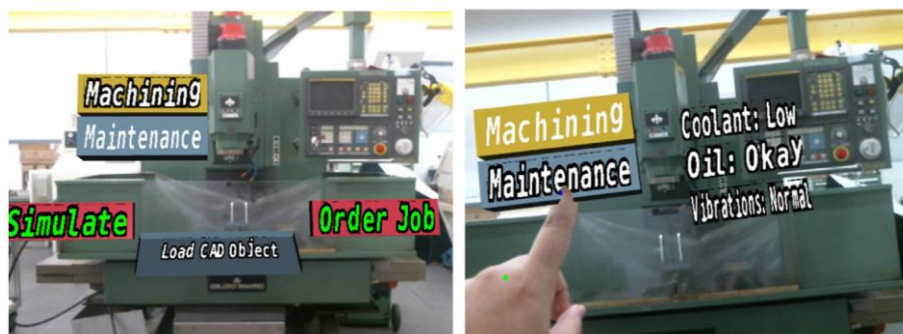
Figure 110: Augmented Reality user interface machining context (left) and maintenance context (right)
