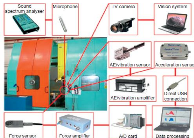
Figure 34: Reconfigurable multi-sensor monitoring system concept (Grzesik, 2017a)
