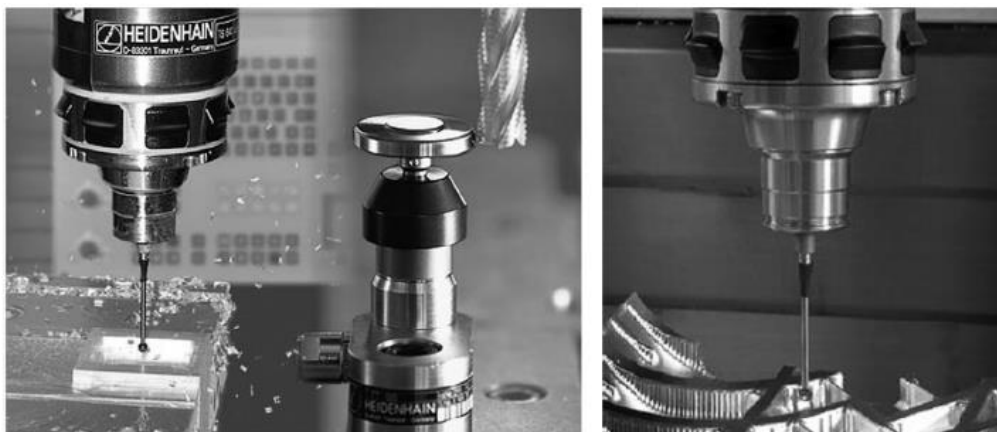
Figure 60: On-machine probing: Workpiece measuring between machining cycles and tool presetting
