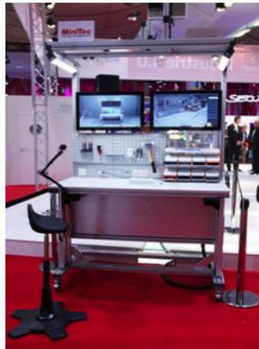
Figure 117: Assistance system and recognition system of a manual assembly workstation
