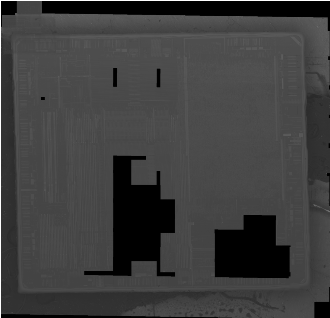
Figure 8.9: Missing tiles in test set 2 stitched with Grid/Collection stitching Fiji-plugin
