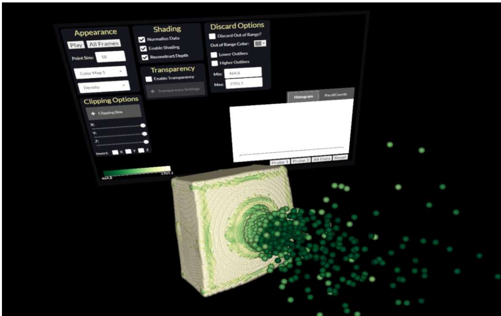
(c) Enabling shading and reconstruct depth. Data is also normalized and point size is increased for better visibility
