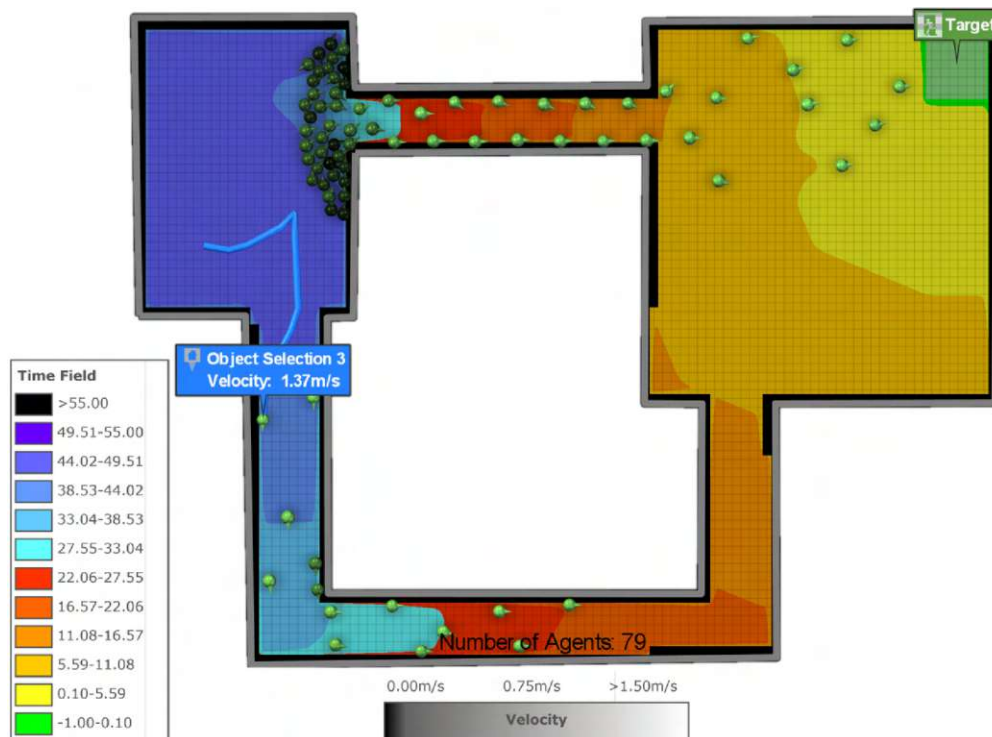
Figure 3.8: The time field of the estimated arrival of the agents. Number of agents is the current number of active agents in the simulation. The path of one agent is traced. It first tried to go through the upper corridor, but then switched to the lower corridor when the congestion formed.
