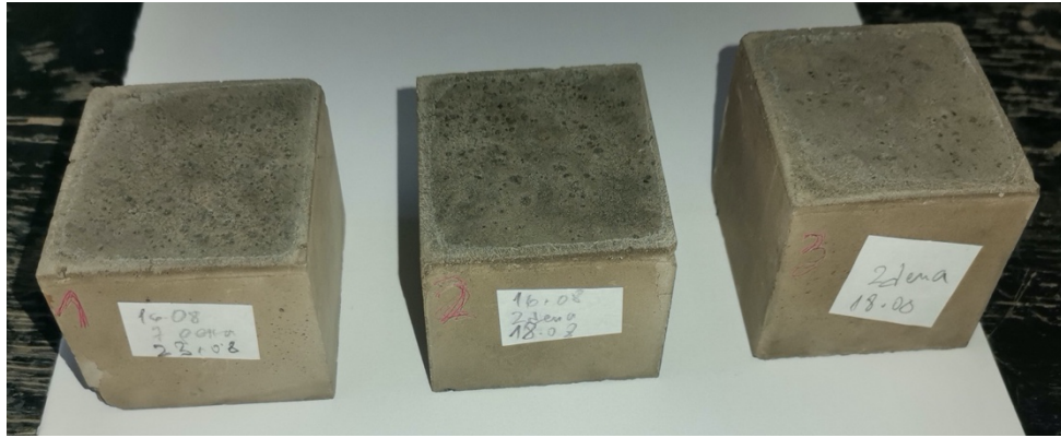
Figure 10. - Samples of alkaline activated materials
