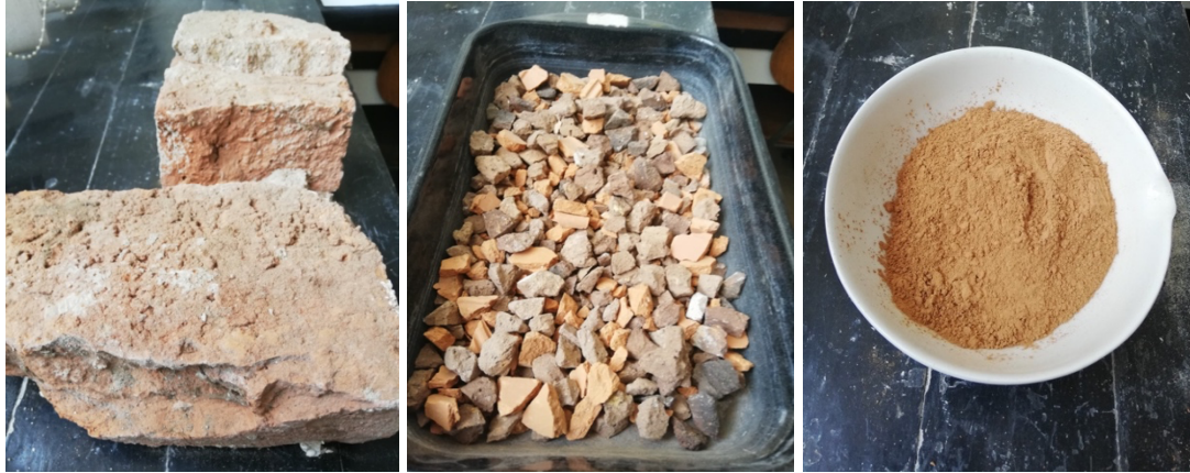
Figure 4. – Preparation the brick waste material
