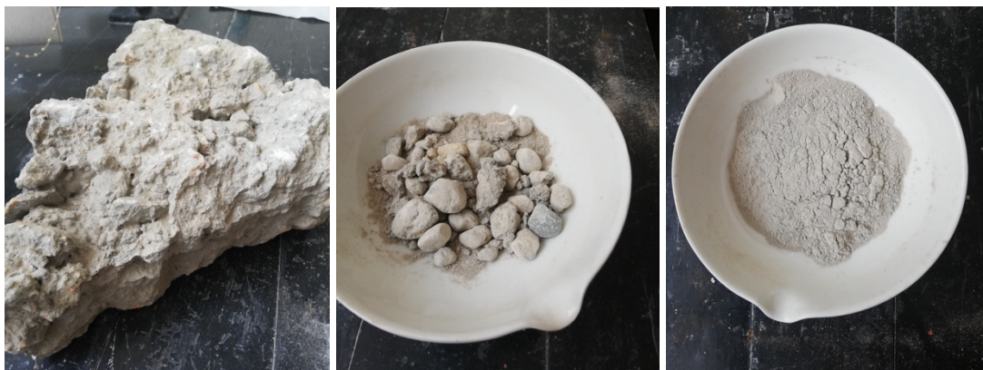
Figure 5. – Preparation the plaster waste material
