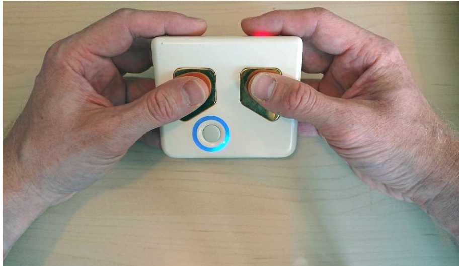
Figure 3.3: SmartPWA device with the left index finger and both thumbs of the user on ECG surface areas and right index finger on PPG surface area. Developed and built by the AIT (Vienna, Austria).
