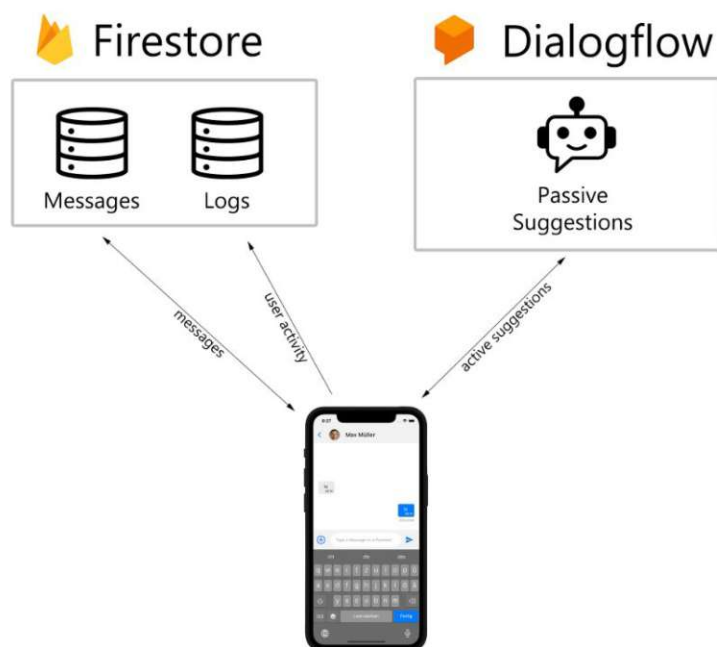
Figure 3.30: Technical architecture of the “Inline“ prototype
