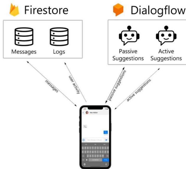
Figure 3.31: Technical architecture of the "Suggestion" prototype
